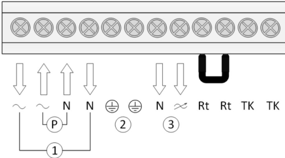
(\*1) Relay connection. There is always 230V between ~ and N when the transformer knob is in one of the positions 1-5.
