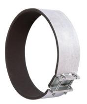
The fan can be connected to duct with mounting clamp MK. The mounting clamp is made of galvanized steel sheet with a rubber seal to fit tightly and absorb vibrations.
