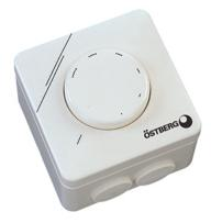
VRS for manual variable speed control of single-phase AC motors. Minimum speed is set by means of a screw under the knob. All single-phase fans from Östberg can be regulated with the VRS controller. The controller is certified and approved as conforming to electrical safety and interference regulations on all markets. Suitable for recessed as well as for surface mounting.
